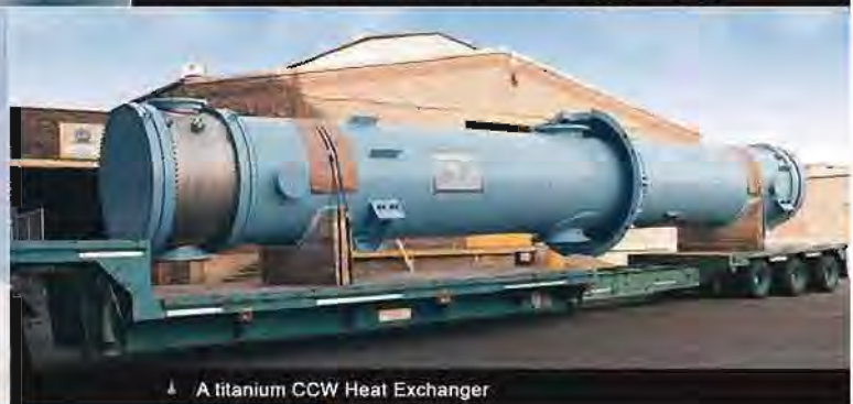
▲ A titanium CCW Heat Exchanger
