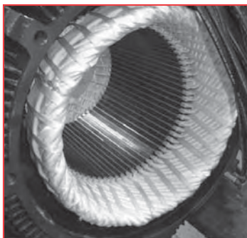
Above: Schulz Technicians using high pressure steam cleaning to decontaminate a 9000 hp rotor. Left: Completed rewind of 150 hp random wound motor pre-vpi.
